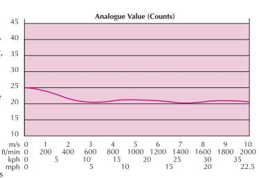
Fig.6 Typical wind speed response - XP95 Ionisation Smoke Detector
